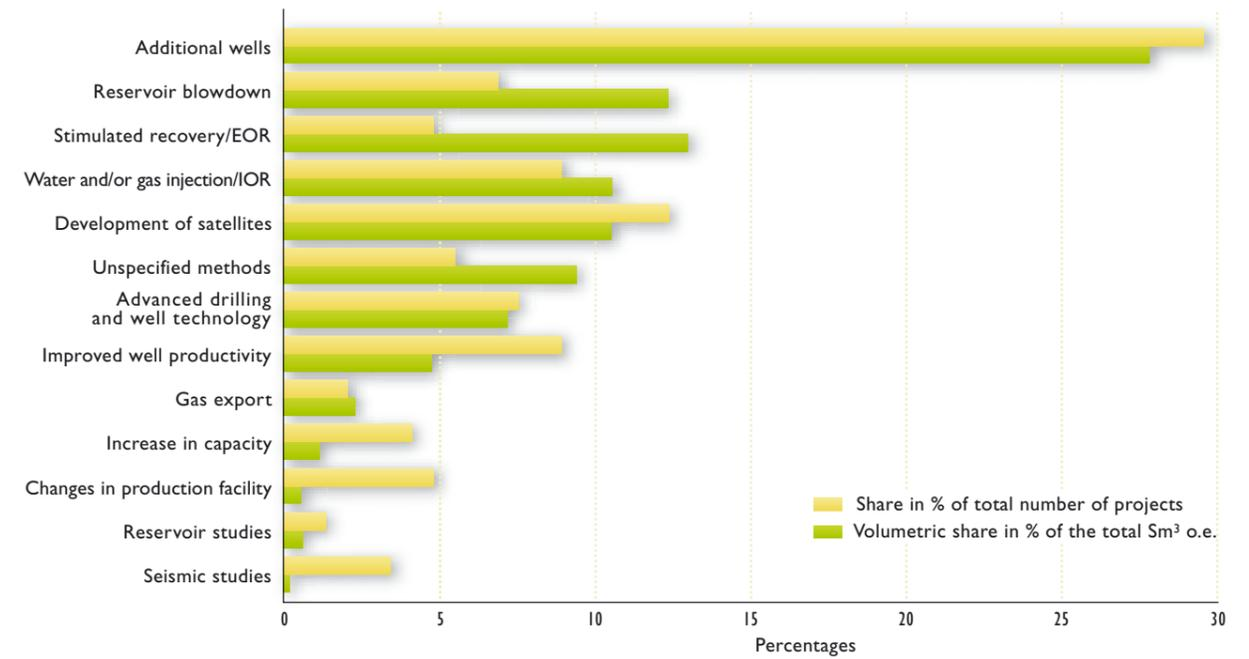
**Figure 5.17** Distribution of the potential for improved recovery from various measures planned on fields in production. Most of the projects and the highest potential volumes concern drilling of additional wells.
