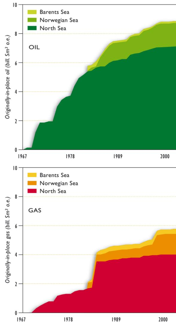
**Figure 2.1** The growth of originally-in-place quantities of oil and gas in the North Sea, the Norwegian Sea and the Barents Sea. The estimate of the in-place petroleum in each deposit may change over time as a result of new mapping and understanding, or because an appraisal well shows that the discovery is larger or smaller than initially assumed. The figure shows the present estimate of the in-place resources.
