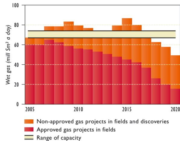
Figure 6.13 Illustration of the capacity situation for the Åsgard transport system. Non-approved gas projects in fields and discoveries include those where a need for transport has been indicated over and above present-day reservations. This applies to the Heidrun, Njord and Åsgard fields, and the 6407/1-2 Tyrhans, 6507/5-1 Skarv, 6507/5-3, 6507/3-3 Idun, 6507/2-2 and 6707/10-1 discoveries.
