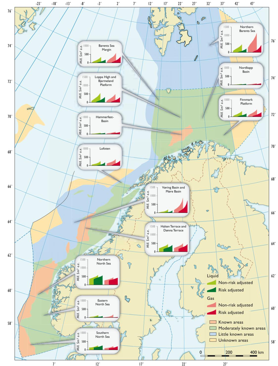
**Figure 3.6** Potential for undiscovered resources in areas of varying maturity. The foreground bars show the expected mean quantities of liquid and gas, respectively, and the uncertainties involved. The bars behind these show the theoretical (non-risk adjusted) basis for the estimates on which the means and ranges of uncertainty are based if all the plays in the area are confirmed.
