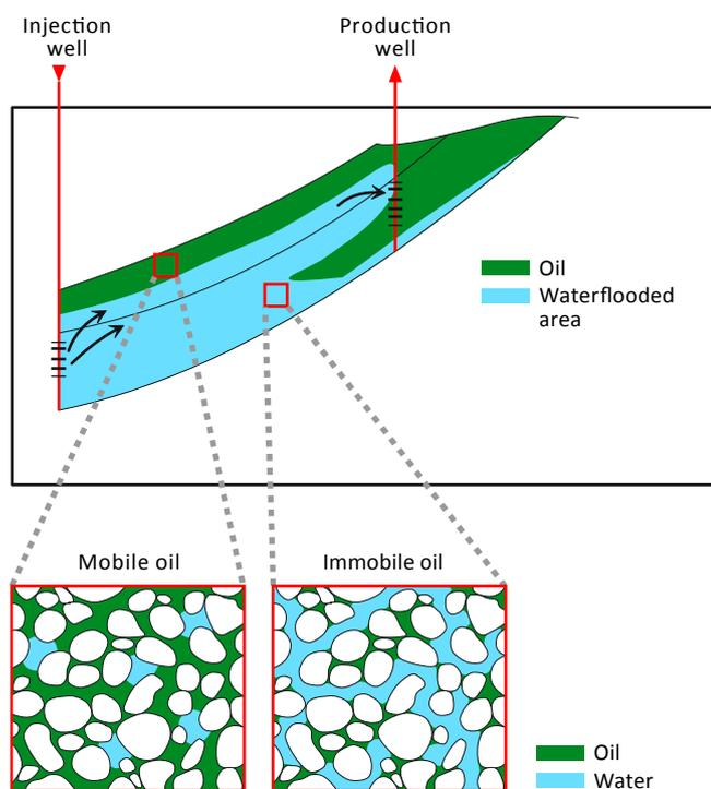
**Figure 2.13** Cross-section of a reservoir showing an example of oil and water distribution after waterflooding, and distribution of the liquids at pore level.
