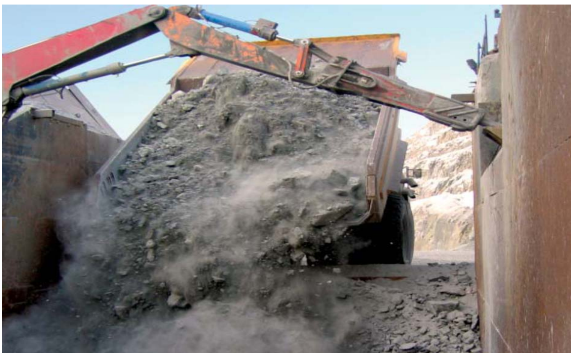
Figur 41. Innlasting i en spindelknuser (gyratory crusher)
