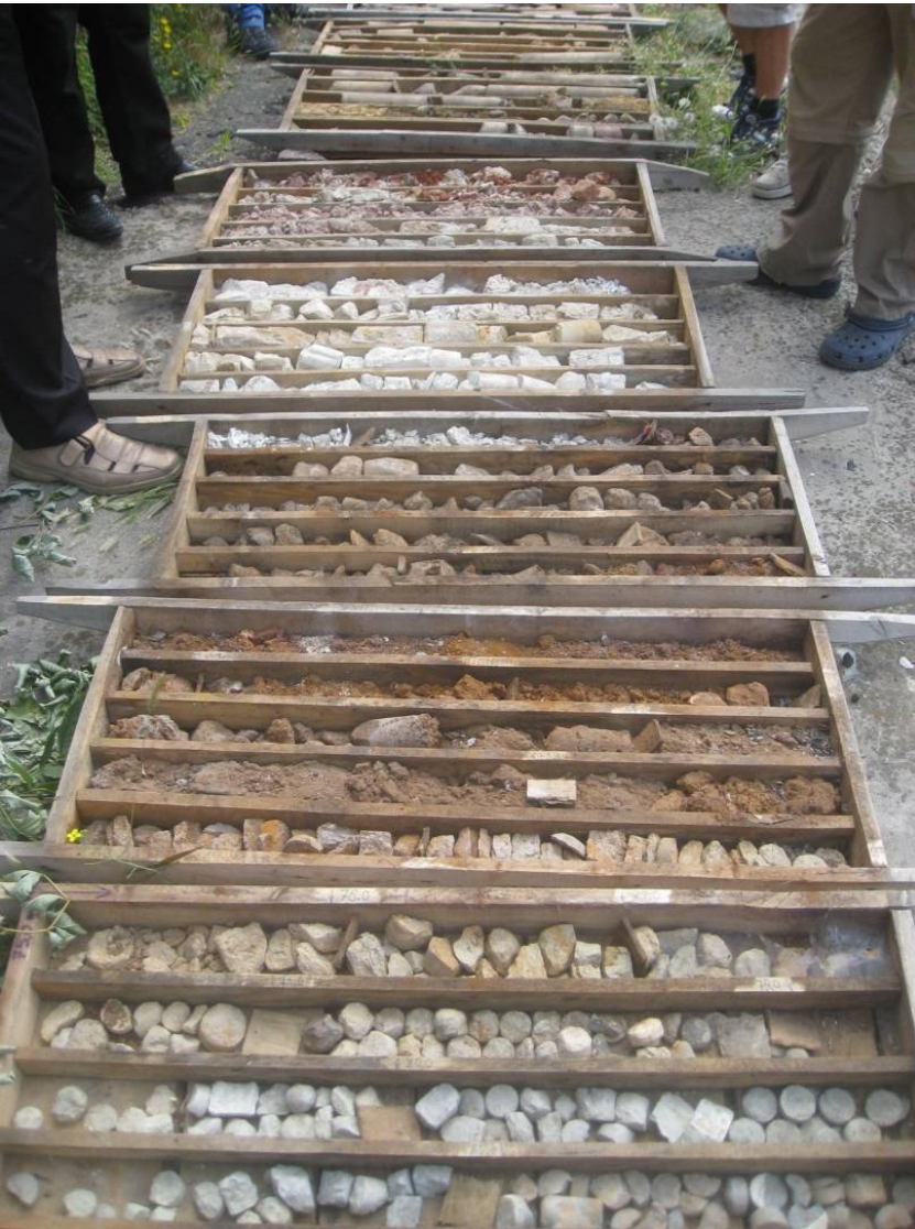
Borehole samples of deep weathering in Ukraine; limonite, silcrete, soap stone and clay containing kaolinite, smectite and hyalite.
