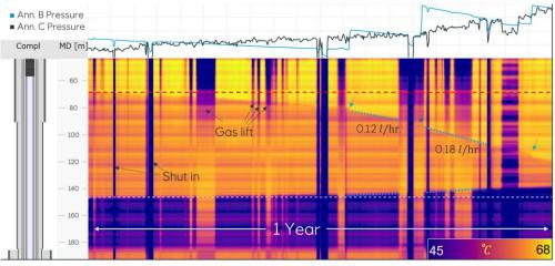
DTS data from a 1-year period recorded in an oil producing well with occasional gas lift.
