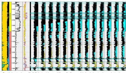
Open hole saturation profile (left), horizontal permeability profile (linear scale), density / neutron logs and saturation profiles from (Fortier, B., et al. SPWLA 65th Annual Logging Symposium, May 18-22, 2024).
