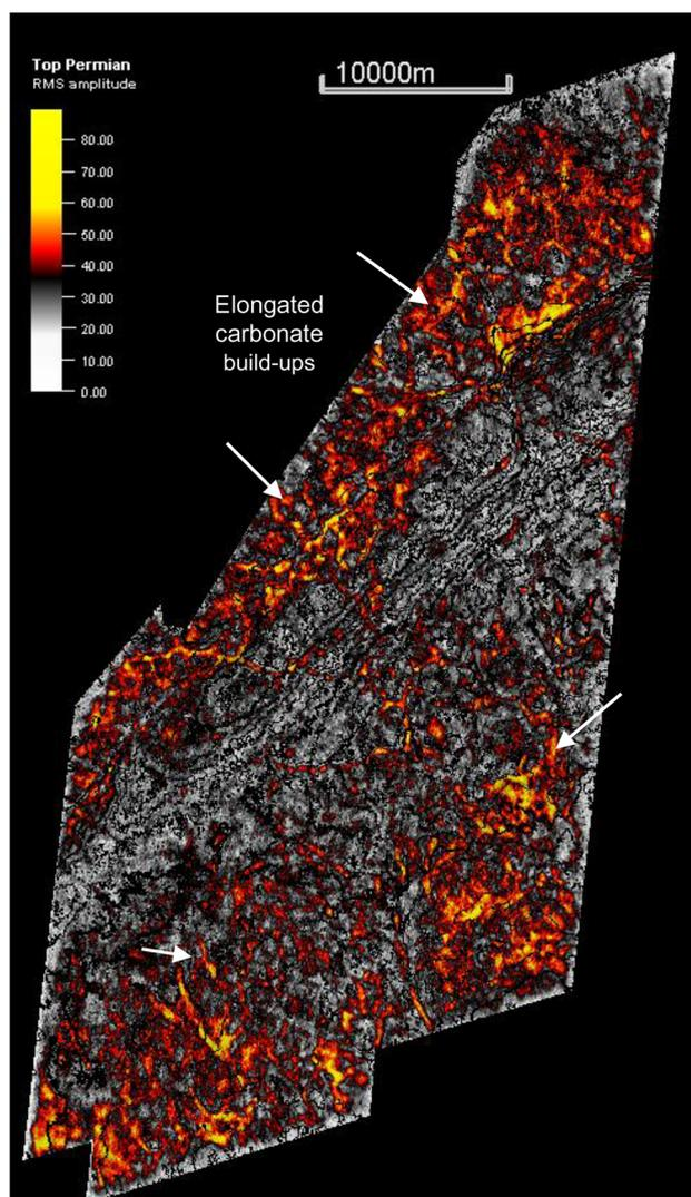
**Fig. 11.** RMS amplitude map from the Top Permian surface on the eastern parts of the Sentralbanken high, showing a network of elongated carbonate build-ups. The location of 3D seismic survey NPD19001 is shown in Figure 2.
