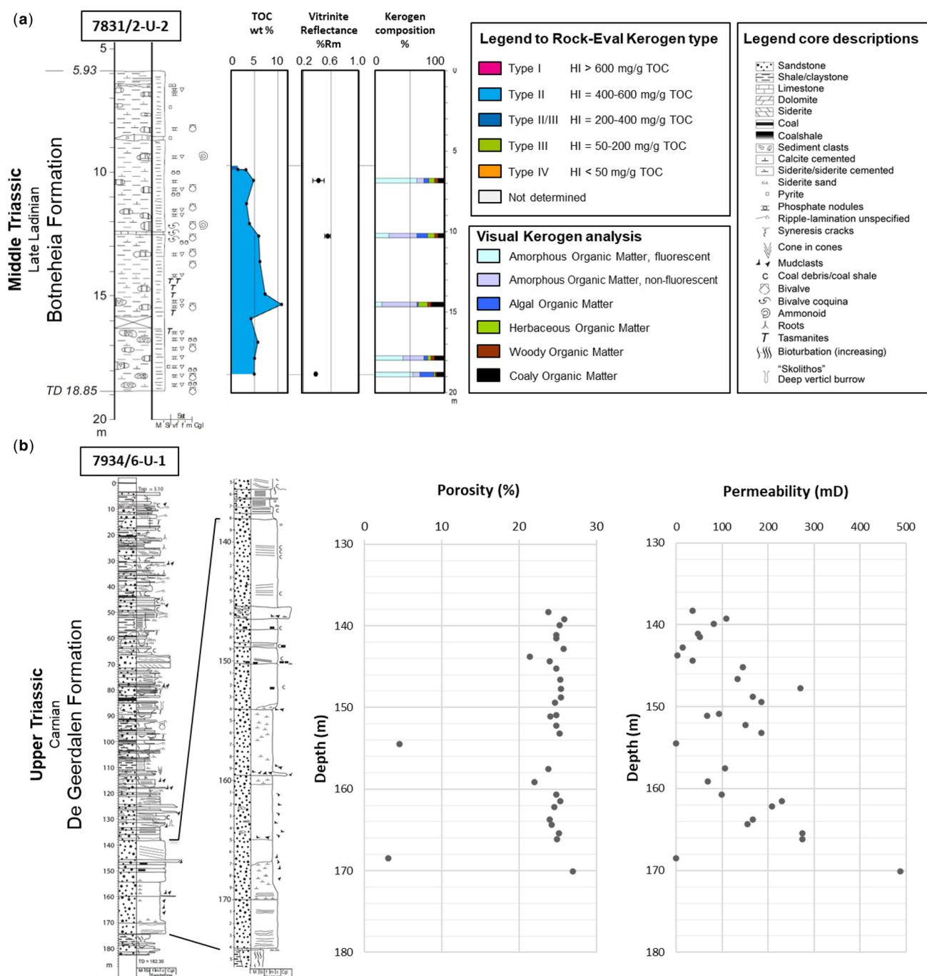
**Fig. 10.** (a) The organic-rich source rock assigned to the Steinkobbe/Botneheia Formation in 7831/2-U-2 on the Kong Karl platform. (b) Channel sandstones with good reservoir properties in core 7934/6-U-1 offshore Kvitøya.
