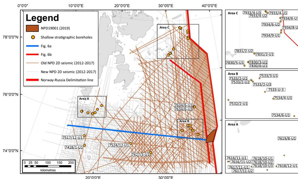
**Fig. 2.** Overview of shallow stratigraphic boreholes and regional seismic data coverage including vintage (grey) and new (orange) 2D surveys in the North Barents CTSE. The brown-filled polygon marks a 3D survey. The regional geoseismic profiles in Figure 6 are also indicated.
