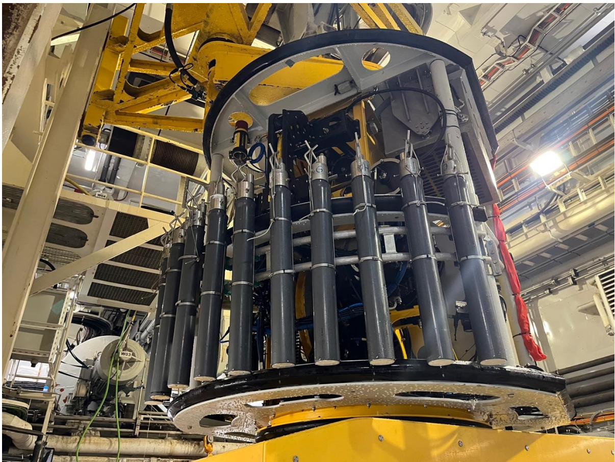
Figure 3: The 10 push cores (A-J) attached to the TMS by metallic hose clamps.
