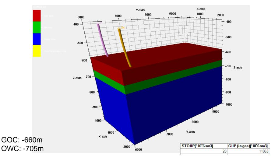
Yellow, horizontal exhaust gas injector, Purple, horizontal oil producer
