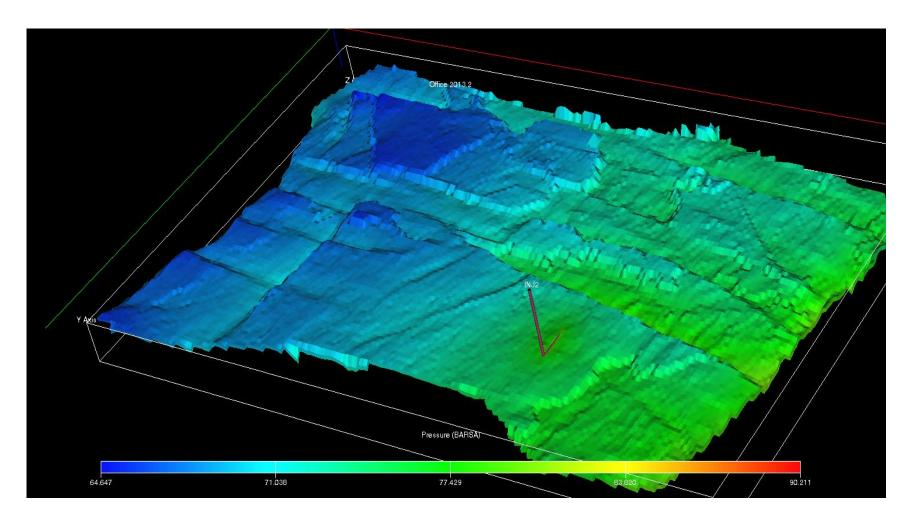
The model of the saline aquifer is based on a real geological case. It is approximately 13x10 km with a reservoir thickness of 10-20 m. Simulations were run with open and closed boundaries.
