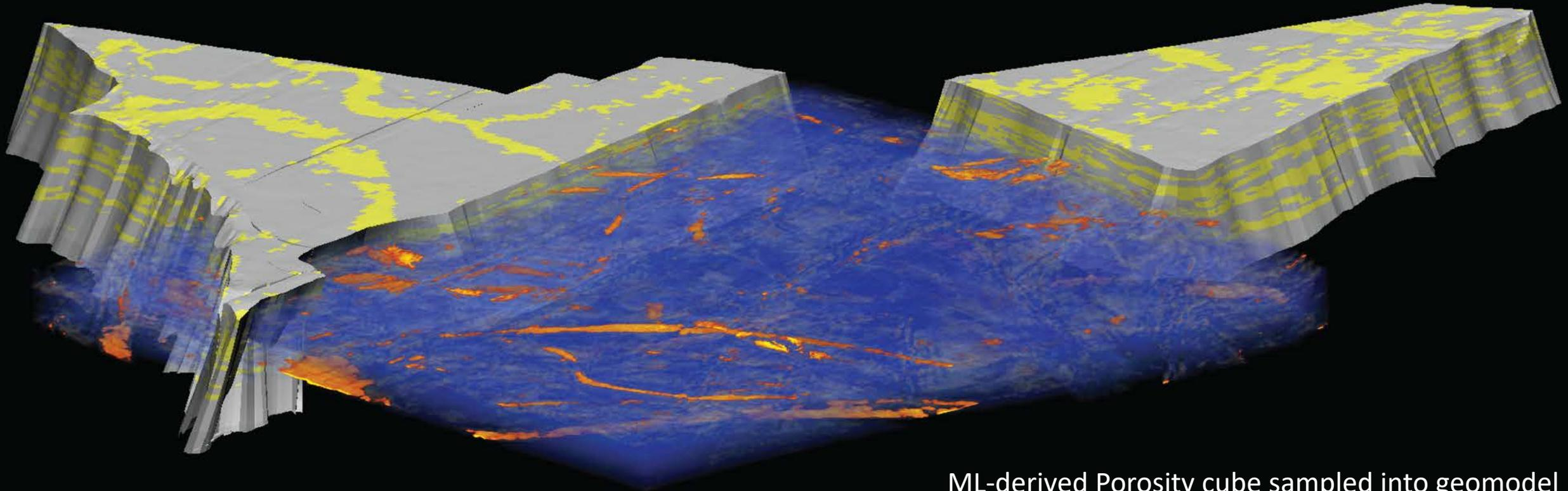
ML-derived Porosity cube sampled into geomodel
