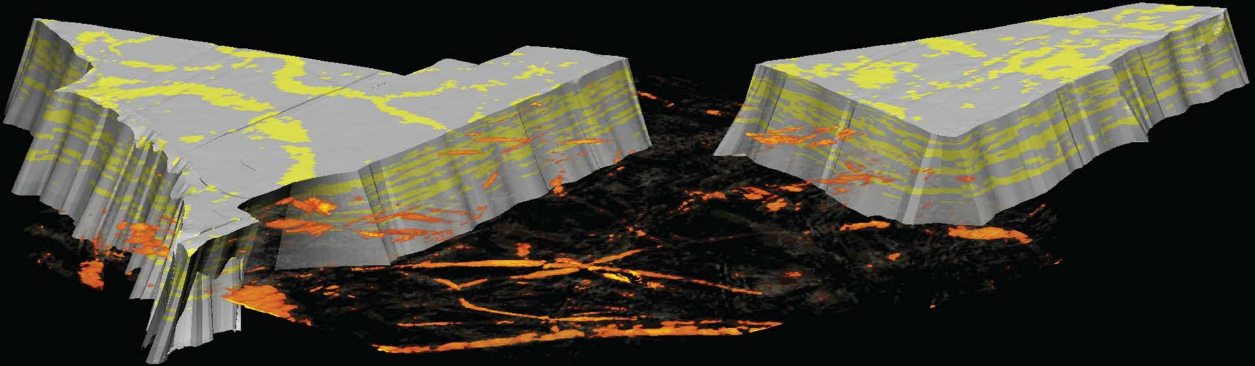
ML-derived Porosity cube sampled into geomodel
