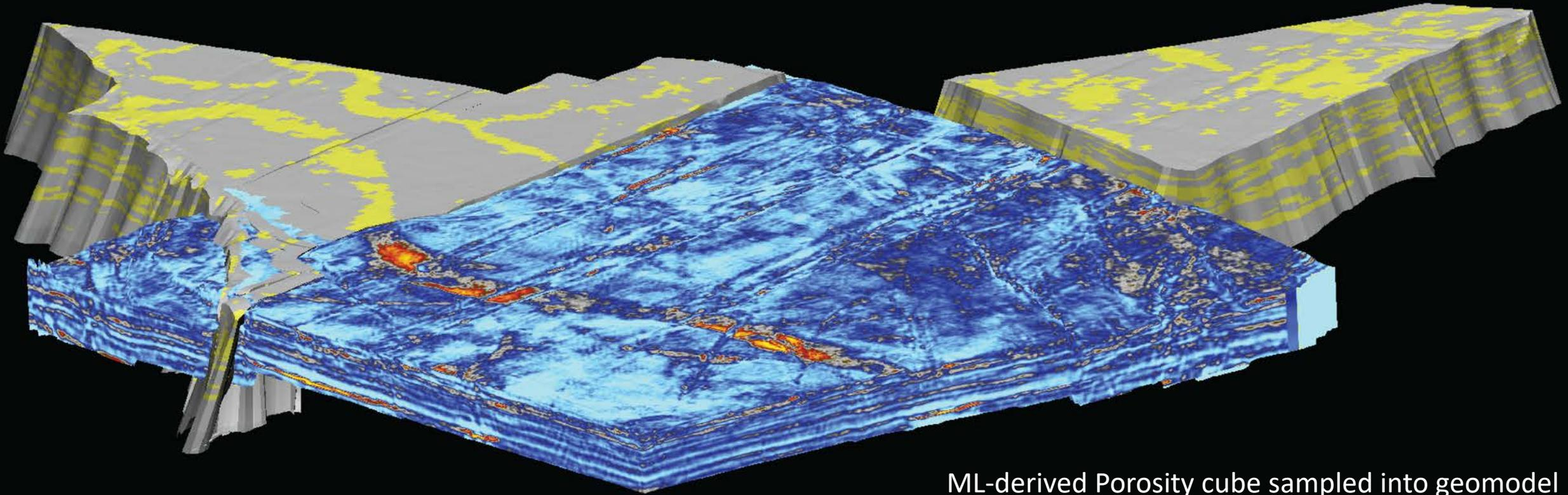
ML-derived Porosity cube sampled into geomodel
