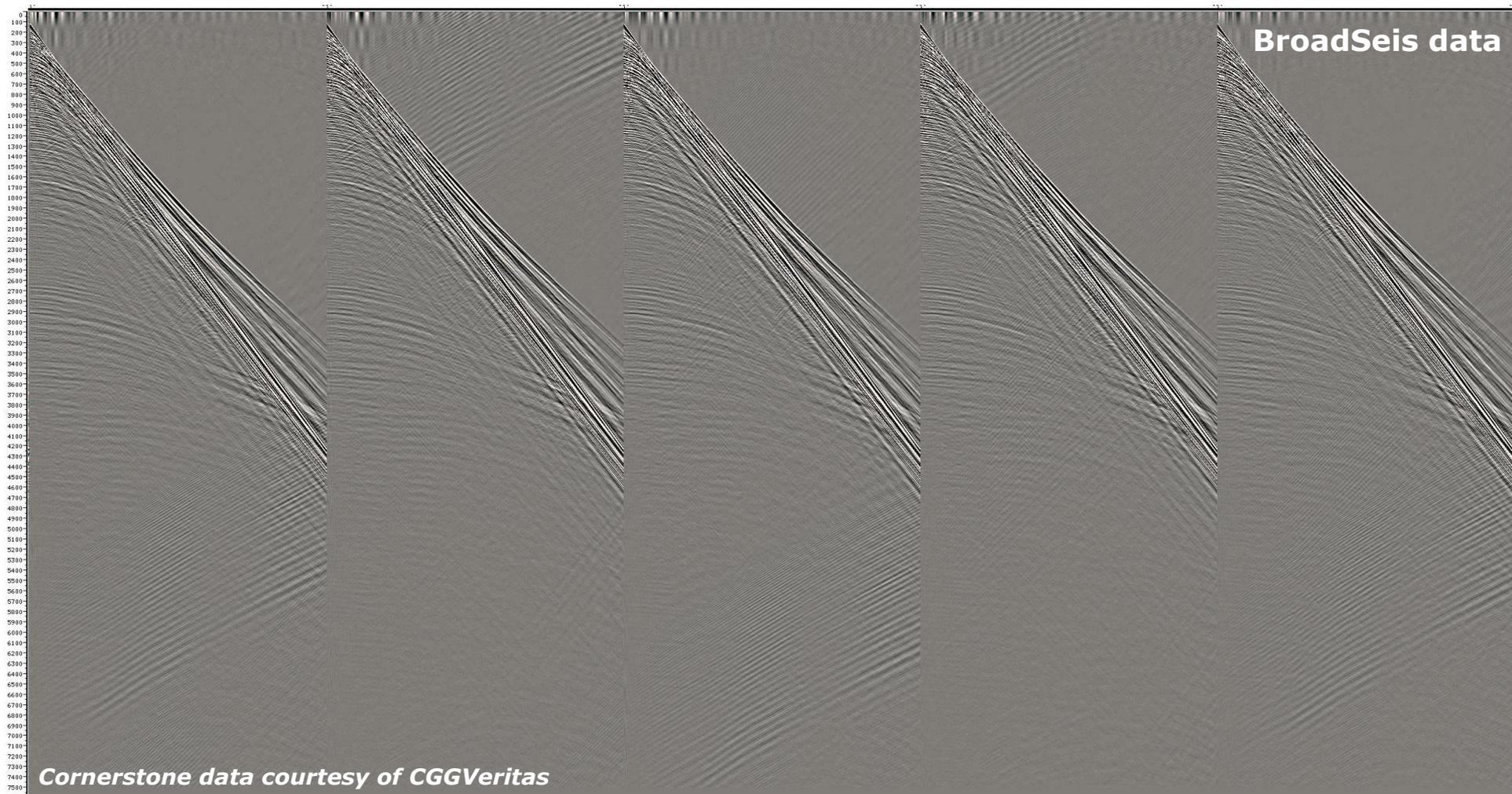
**6 km Variable Streamer Depth from 5m to 50 m**
