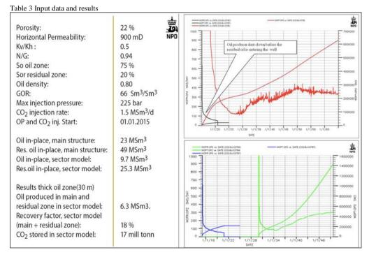
Figure 12a Oil production profiles with sensitivities (Red: base case model with 30 m oil zone. Black: sensitivity with 3 m oil zone.
