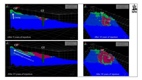
Figure.11 Profiles through the  $CO_2$  injector (GI) and the oil producer (OP), showing distribution of  $CO_2$  (red), oil (green) and water (blue) 3 and 25 years after the injection start. The maps to the right show the distribution of the  $CO_2$  plume. North is down to the left.
