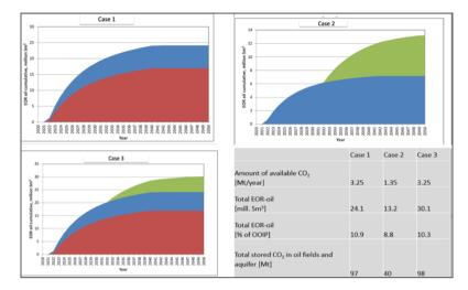
Figure.5 The EOR effect from three oil fields with injection of 1-3 Mt CO2 annually for EOR and storage, over 30 years.
