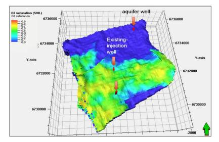
Figure 7 Reservoir model with different location of CO2 well injection
