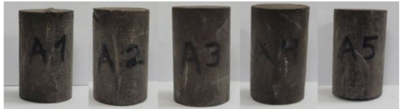
System A – After 6-months in carbonic acid
