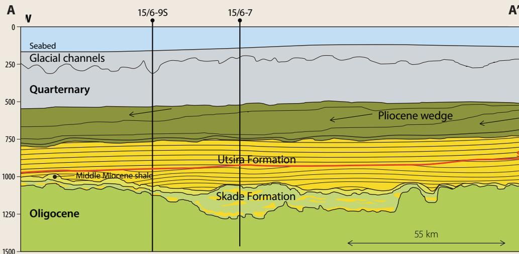
The Skade Fm, Lower Miocene, consists of marine sandstones (mainly turbidites) deposited over a large area of the Viking Graben (From 30/5-2 in the north, to 15/6-7 in the south). The maximum thickness exceeds 300 m and decreases rapidly towards the south and east, where the sands terminate towards large shale diapirs.
