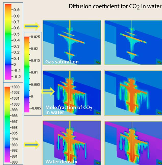
Long term effects of CO<sub>2</sub> injection for two alternative values of diffusion coefficient.
