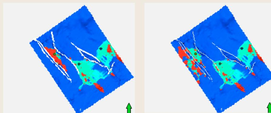
CO<sub>2</sub> distribution after 1000 year from injection start. With closed faults (left), and open faults (right). A part of the CO<sub>2</sub> migrates through the faults to the west.
