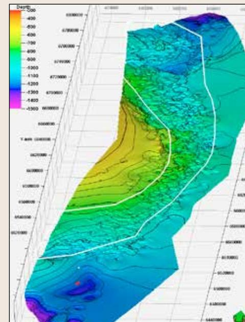
Top of Skade Formation. The white polygon indicates area which may be favorable for CO<sub>2</sub> storage. Red dot shows Sleipner injection area. The grid squares are 20 km x 20 km.
