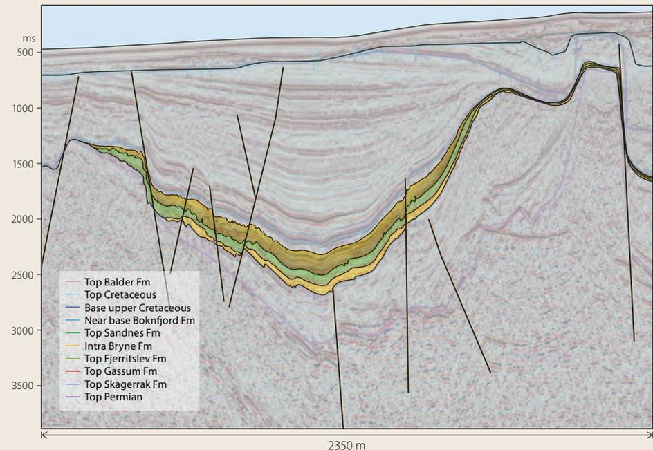
Seismic section across the Farsund Basin. The Gassum aquifer is located between the red and the dark blue horizon at the base of the Jurassic section.
