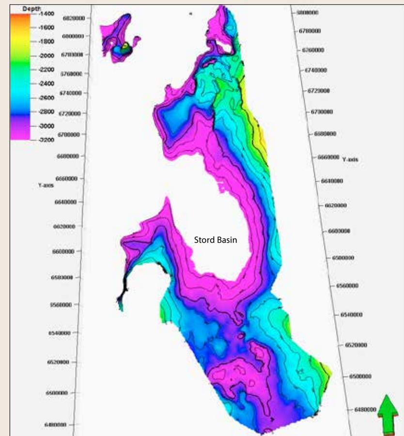
The top of the Statfjord Formation above 3500 m. The Tampen area to the NW was not included in the volume calculations.
