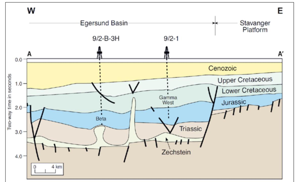
Geoseismic cross section in the Egersund basin.
