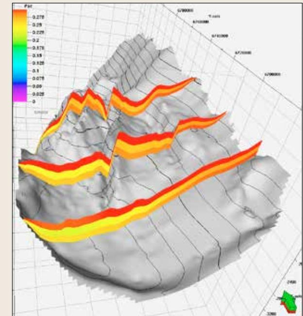
Cross sections showing the Krossfjord, Fensfjord and Sognefjord formations with modelled porosity values above the Top Brent surface within the Sognefjord Delta.
