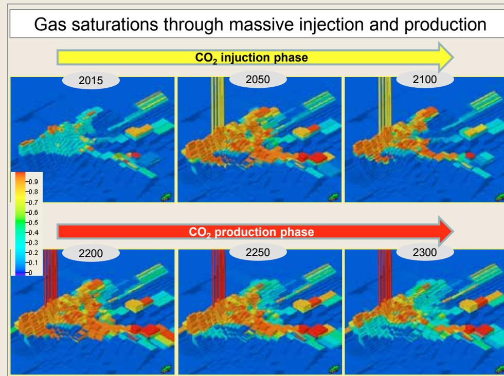
The figure shows the gas saturation during the injection and production. Some of the CO<sub>2</sub> will be trapped behind the waterfront due to relative permeability effects. No diffusion is assumed in this case. 50 MSm<sup>3</sup>/d. CO<sub>2</sub> injection during 2015-2100 and reproduction from year 2200 at 5 MSm<sup>3</sup>/d.
