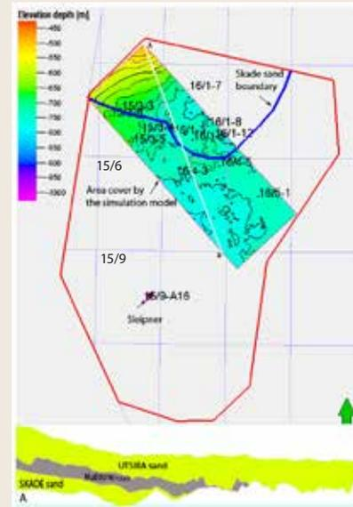
Red boundary defines the southern depocenter of the Utsira Formation. Skade Formation thins rapidly towards south and east, and is only observed as a few meters thick in well 15/6-7. The simulation model covers an area of 1600 m<sup>2</sup> within the southern depocenter.
