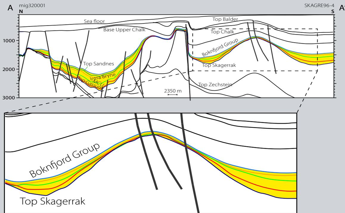
The enlarged rectangle shows the Jurassic section within a salt-induced structure. MCU is the base of the Bryne Formation.
