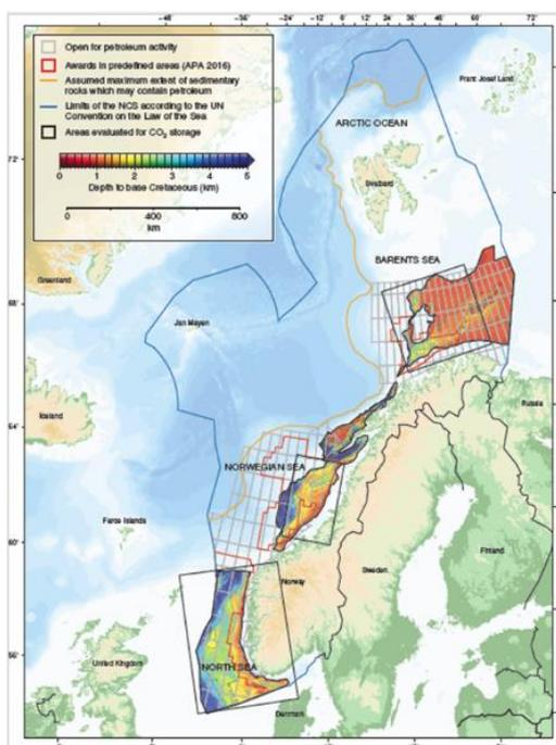
Figure2 Areas offshore Norway evaluated for potential CO<sub>2</sub> storage.
