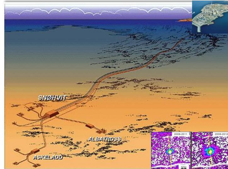
**The Snøhvit gas field** in the Barents Sea. The well stream, with natural gas, CO<sub>2</sub>, NGL and condensate, is transported in a 160-kilometre pipeline to the facility onshore. The gas is processed and cooled down to liquid natural gas (LNG). The CO<sub>2</sub> is separated and returned to the field by pipeline for reinjection into a geological formation.
