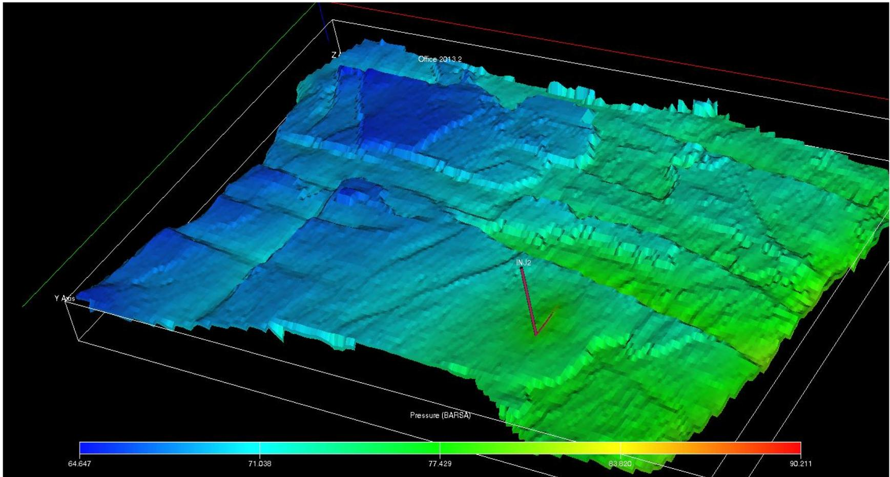
The model of the saline aquifer is based on a real geological case. It is approximately 13x10 km with a reservoir thickness of 10-20 m. Simulations were run with open and closed boundaries. The colours show initial pressure, which is hydrostatic and varies from 65 to 75 bar, 70 bar in the well position. Average reservoir properties: Porosity 20 %, permeability 400 mD.
