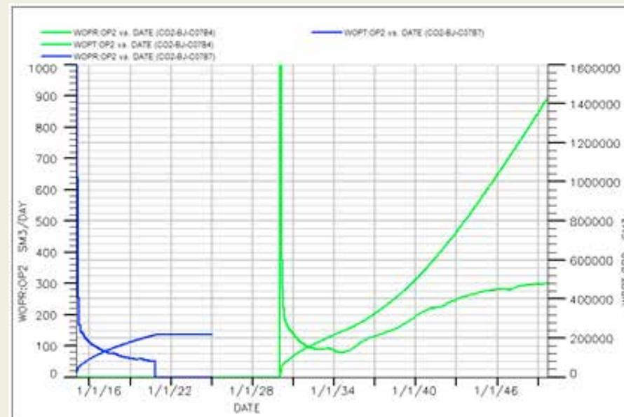
Oil production starts 15 years after CO<sub>2</sub> injection ( Blue: CO<sub>2</sub> injection and oil production startup simultaneously. Green: Delay of production 15 years after CO<sub>2</sub> injection startup.
