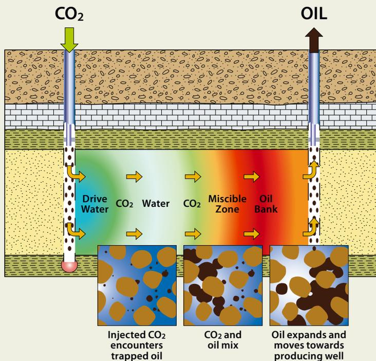
Cross section of a reservoir with CO<sub>2</sub> WAG
