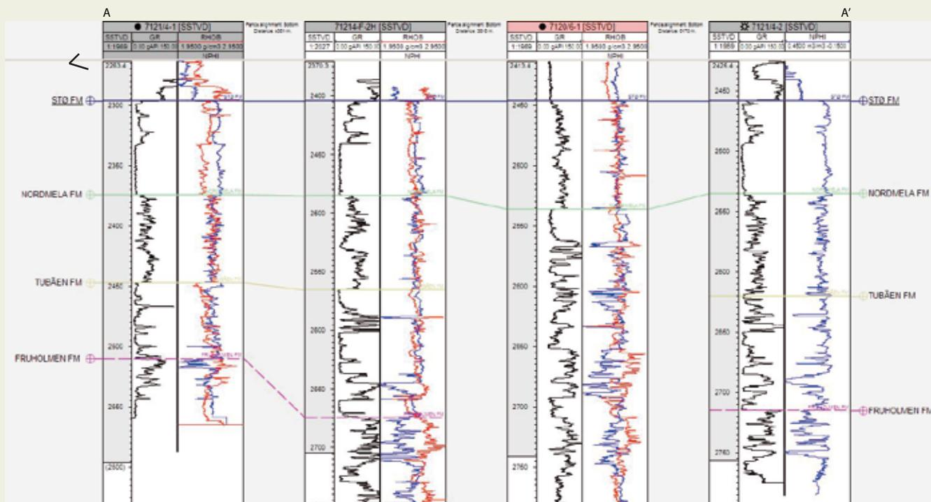
Log correlation panel with gamma and neutron/density, flattened on the Stø Fm. Location of profile is shown in the Stø Fm thickness map.
