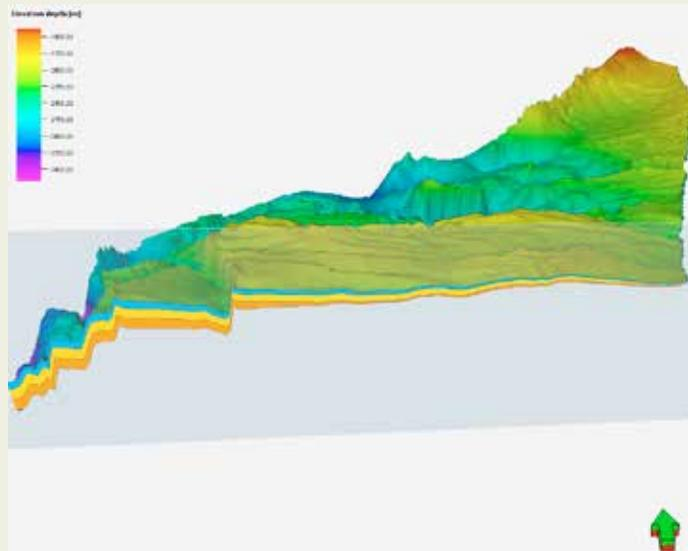
W-E cross section through the Hammerfest Basin 3D geological model, showing the Stø, Nordmela and Tubåen aquifers in blue, yellow and orange respectively.
