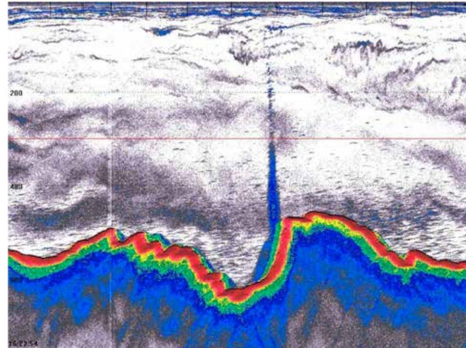
*Detection of gas bubbles by echo sounder systems. The figure shows the acoustic signature generated by CO<sub>2</sub> bubbles being naturally released from the Jan Mayen vent fields. The CO<sub>2</sub> bubbles are here seen as a blue flare that rises around 500 metres from the seafloor through "clouds" of plankton in the water column.*
