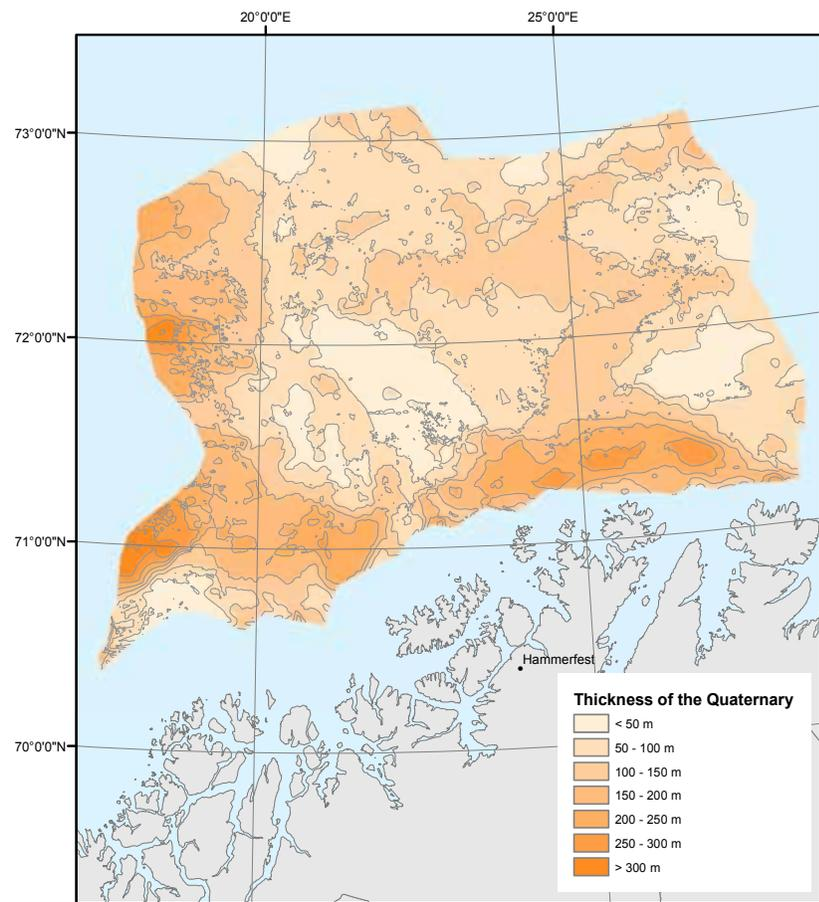
Thickness map of Quaternary in the Barents sea. During the last 2.5 m years glaciers and cold climate dominated in the region, eroding the remnant highs offshore Finnmark and Northern Troms.
