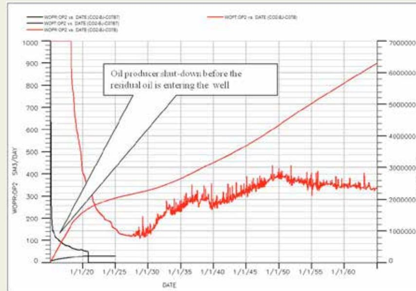
Oil production profiles with sensitivities (Red: basecase model with 30 m oil zone. Black: sensitivity with 3 m oil zone. Oil production and CO<sub>2</sub> injection start 01.01.2015)
