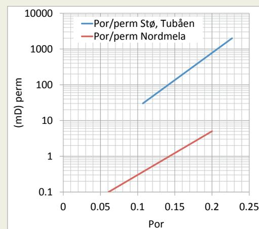
Porosity / depth and porosity / permeability plots based on core and log data from the Hammerfest Basin.
