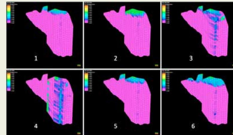
CO<sub>2</sub> plume x-z cross section (J=49) after 1000 yrs.
