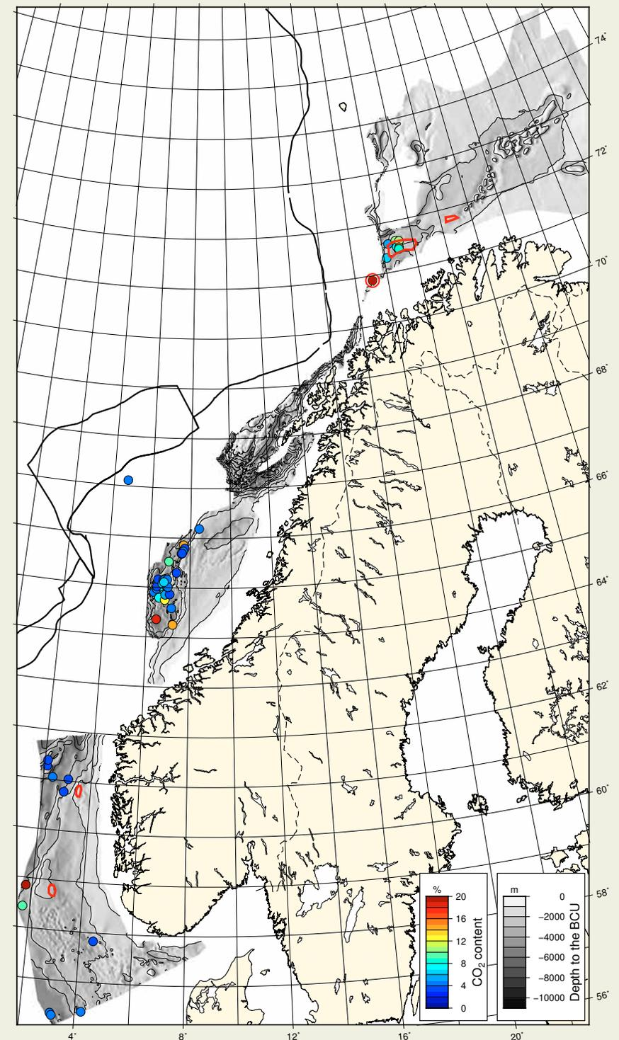
Map of Base Cretaceous unconformity showing location of exploration wells where the measured CO<sub>2</sub> concentration in natural gas exceeds 3 %. 7019/1-1 is marked by a red ring. Residual oil zones are indicated by red lines.
