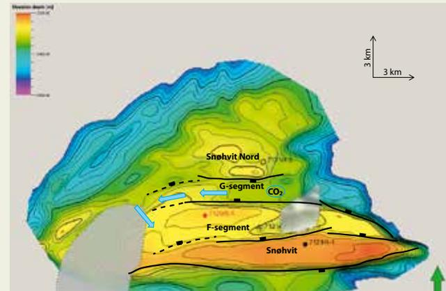
Stø depth map where blue arrows illustrate a possible CO<sub>2</sub> migration after injection in the G segment. Black solid lines illustrate faults with big throw, while black dotted lines indicate where the throw dies out. Grey polygons show location of shallow gas.
