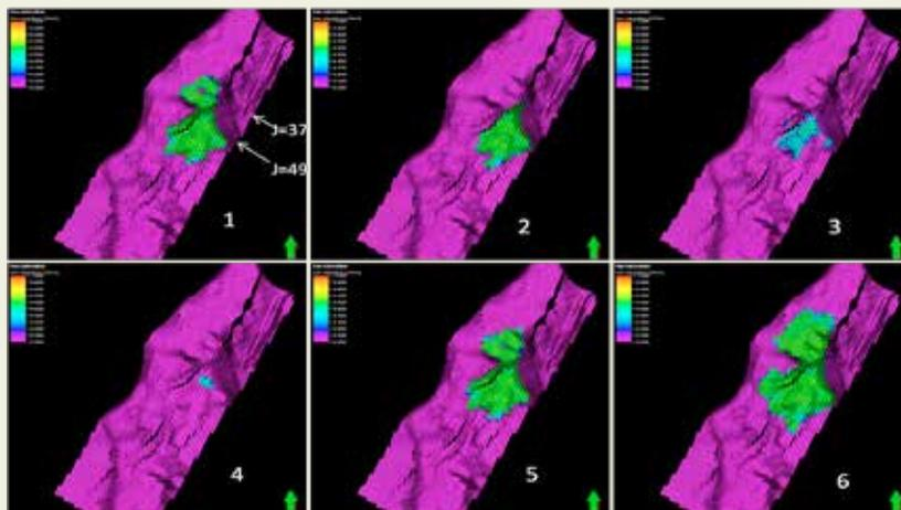
CO<sub>2</sub> plume top reservoir end of injection (50 yrs)
