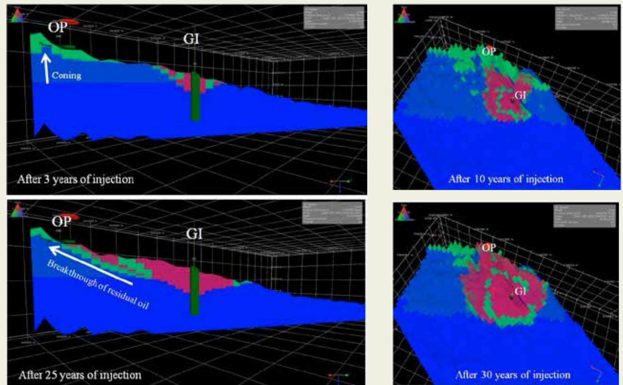
Profiles through the CO<sub>2</sub> injector (GI) and the oil producer (OP), showing distribution of CO<sub>2</sub> (red), oil (green) and water (blue) 3 and 25 years after the injection start. The maps to the right show the distribution of the CO<sub>2</sub> plume. North is down to the left.
