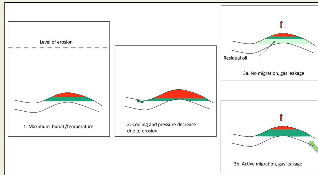
Hypothesis for formation of residual oil zone by natural gas seepage. After maximum burial the rate of seepage of gas is greater than the rate of migration of hydrocarbons into the accumulation. Consequently fluid contacts move upwards. Residual oil (light green) is formed where water replaces oil in the initial oil zone (green).
