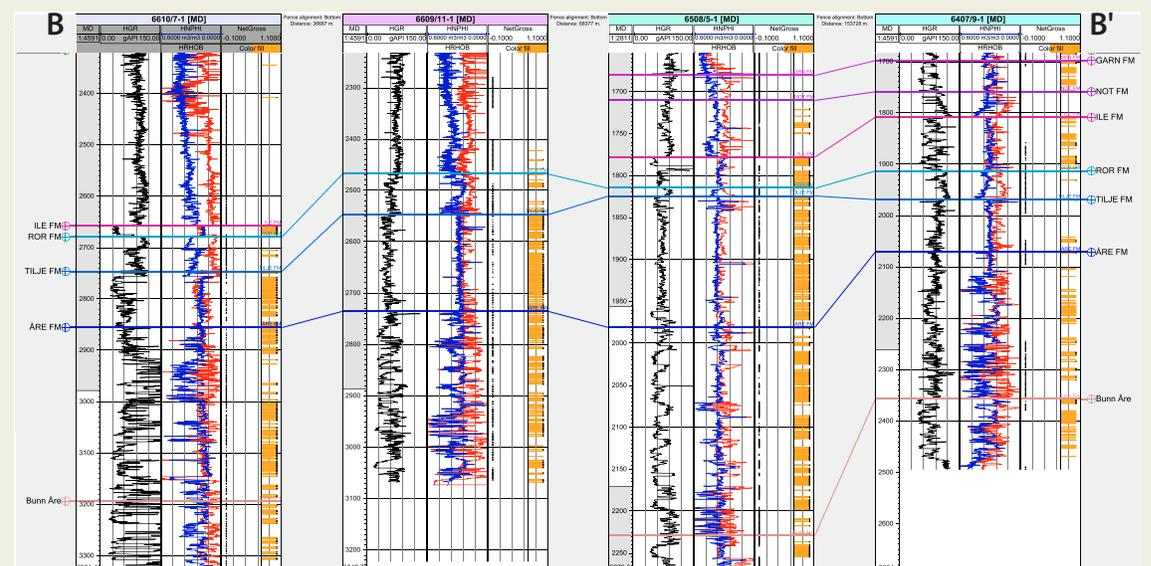
Log correlation panel with gamma, porosity density and calculated net/gross. Layout showed in Garn porosity map.
