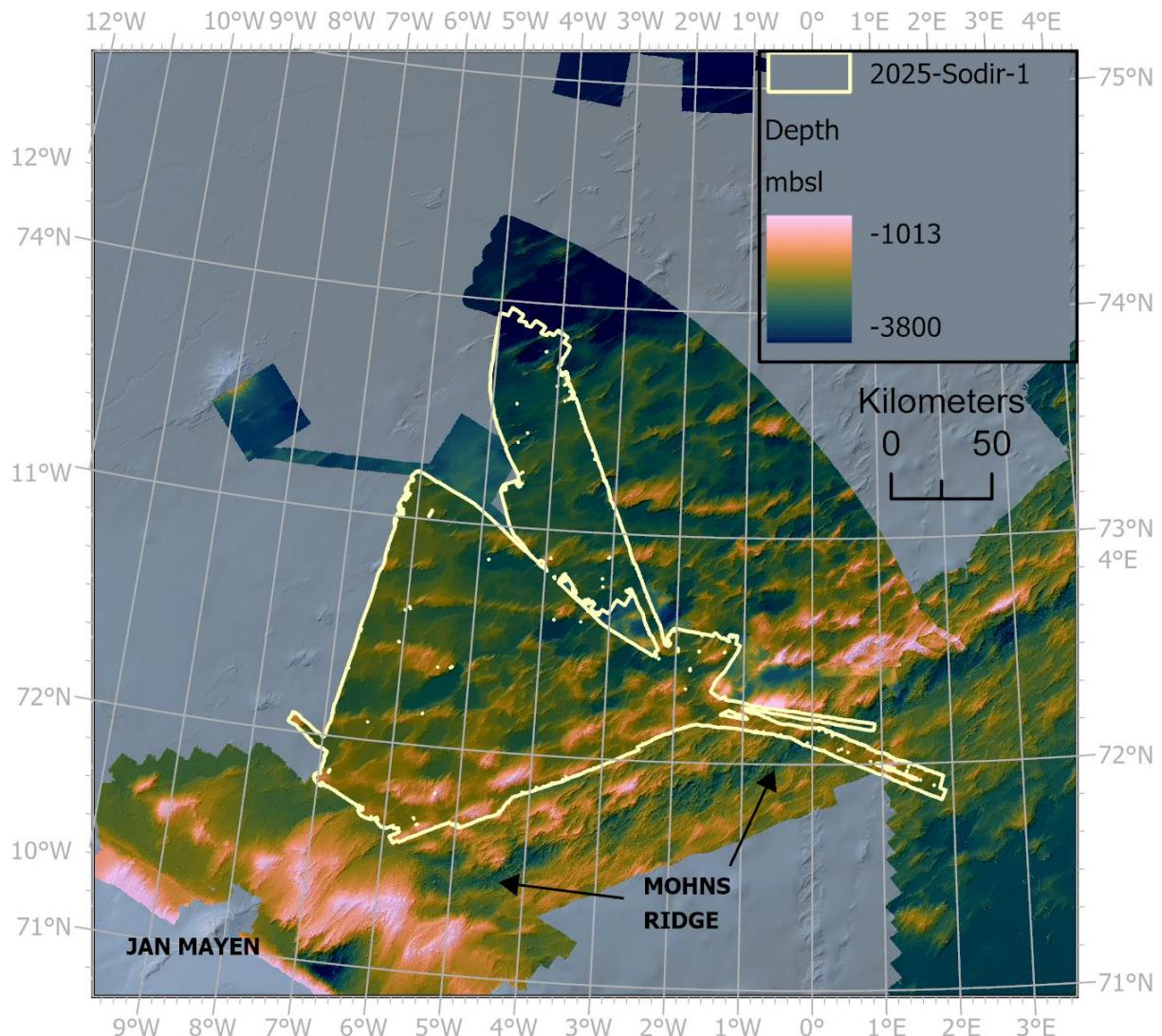
Figure 2: A map displaying an overview of multibeam (MB) data coverage in the region. MB data from survey “2024-Sodir-01” is combined with MB data from other Mareano cruises (see Figure 1), with the current survey outlined in yellow.
