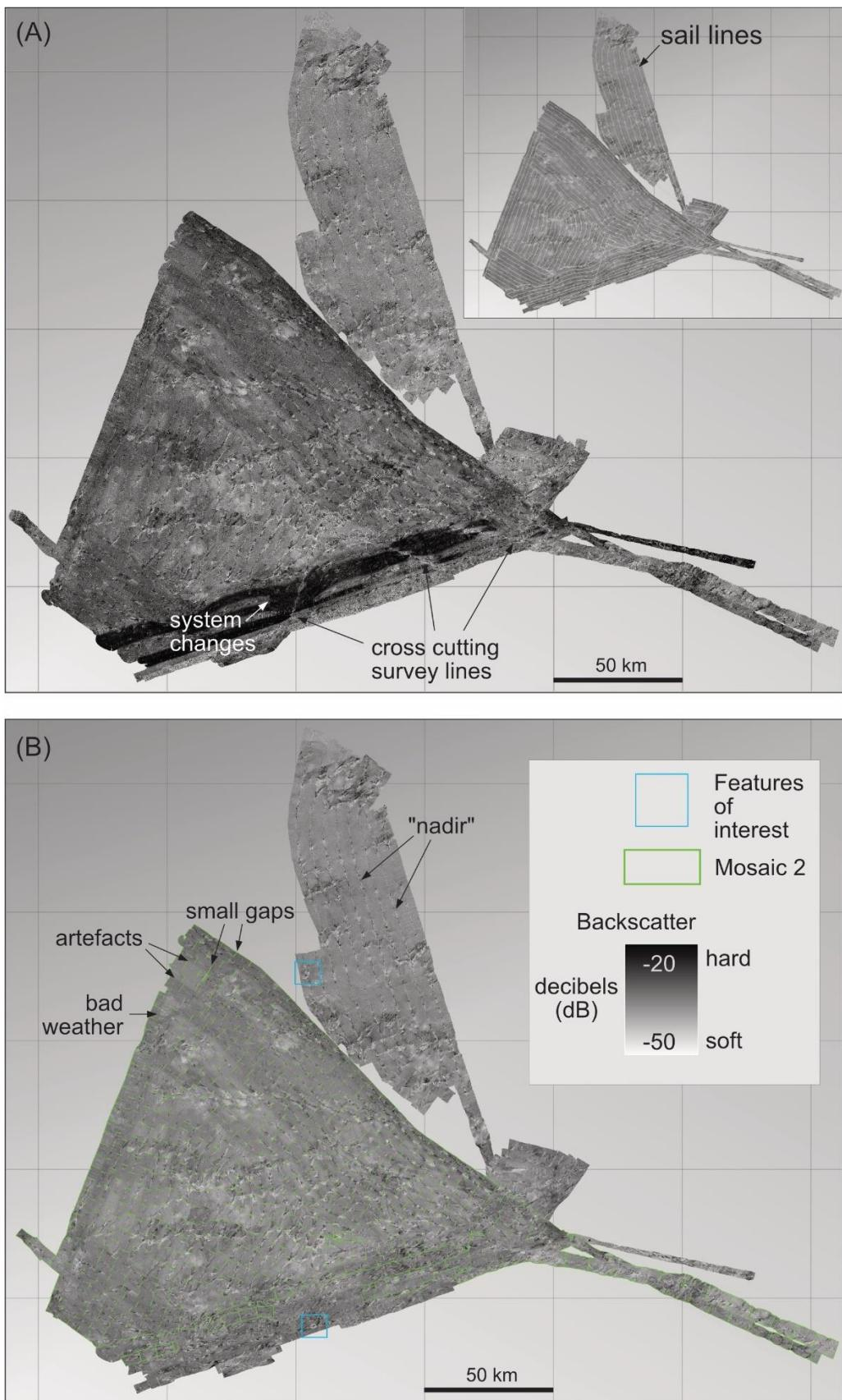
Figure 3. (A) The unprocessed backscatter mosaic, and sail lines shown in insert; (B) The processed backscatter mosaic with the dB range shown for the largest mosaic-2 (green polygon) and features of interest (Figure 5).
