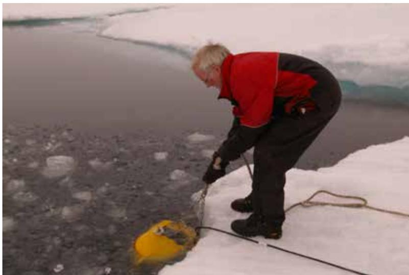
**Data acquisition.** Yngve Kristoffersen deploys hydrophones to pick up seismic signals. About 1 000 kilometres of such data were acquired during the expedition. (Photo: Audun Thølfesen)
