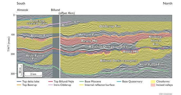
**Profile 1:** North-south trending seismic section from central Jytland, Denmark, showing alternating delta progradation and marine deposits. Note the sand-rich delta lobe deposits indicated in yellow. Fluvial incised valley fill is shown in orange. This pattern characterised the Norwegian-Danish Basin during the Early Miocene. The Middle-Late Miocene was dominated by marine shelf deposits (see also Map 1 for location, modified after Eidvin et al. 2010).
