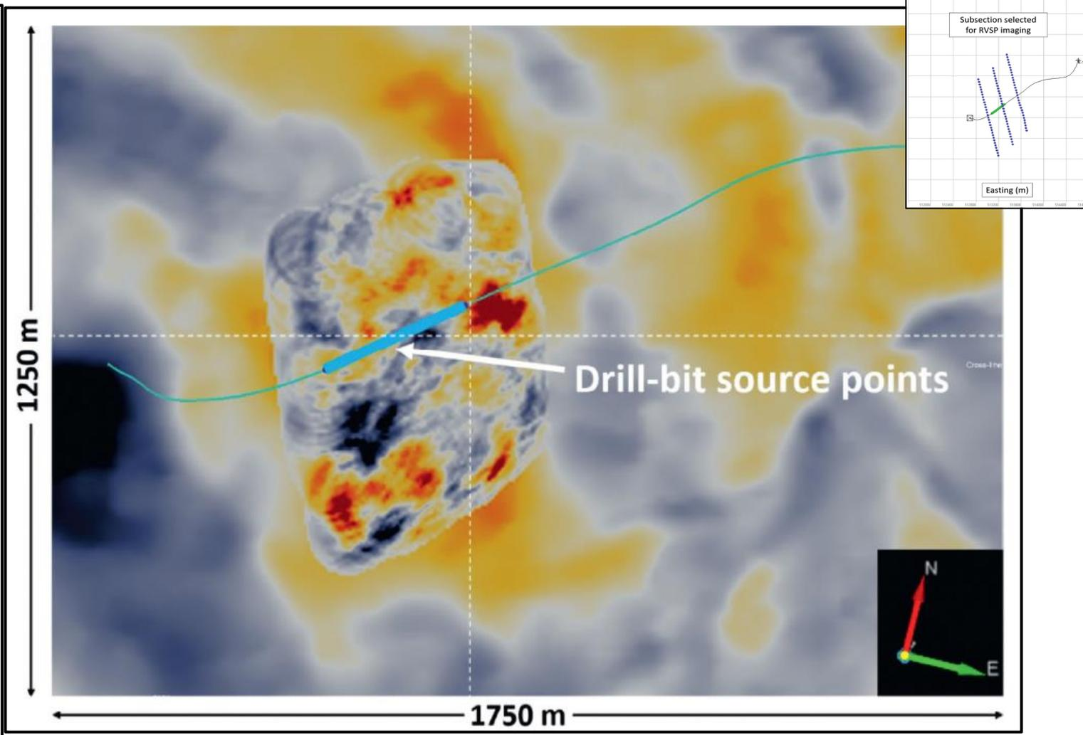
**Figure 7** Depth slice of the spliced image at a depth of 2456 m, illustrating the lateral extent of the 3D RVSP image in relation to the well path. Dashed white lines indicate the location of the inline and crossline slices shown in Figure 8. We observe a good correspondence between the 3DRVSP and the background surface seismic image.
