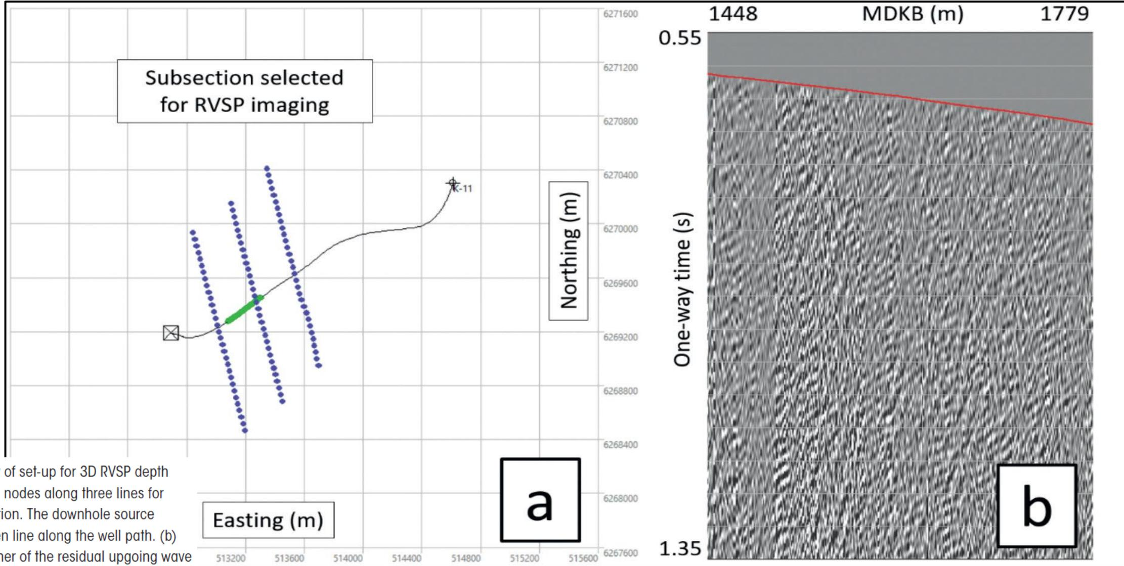
**Figure 5** (a) Map view of set-up for 3D RVSP depth imaging. We select 91 nodes along three lines for processing and migration. The downhole source array is shown as green line along the well path. (b) Common-receiver gather of the residual upgoing wave field input to migration.
