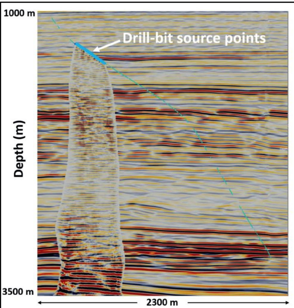
**Figure 6** Seismic depth section along the well path with the corresponding line of the 3D RVSP image spliced in. The well path is indicated by the cyan line with the downhole source array highlighted by light blue thick line.
