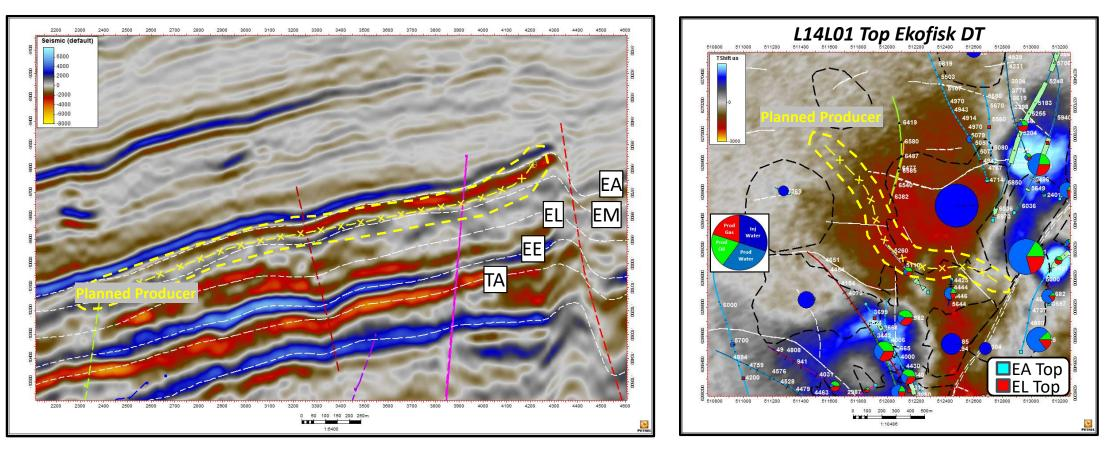
RFT pressure points are white annotations. EA Fm water front polygons are dashed black polygons. Produced and injected volumes per well in the period shown as pie/slice charts on middle perforation
