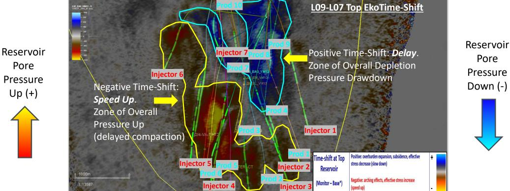
A negative (-) Time-Shift indicates a tightening (speed-up) of the overburden in response to overall reservoir pressuring up (delayed compaction)
