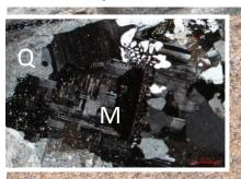
Medium grained red granite, locally fine grained or pegmatitic
