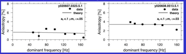
Reservoir: Frequency dependence suggests fractures of ~1m scale, in agreement with outcrop and core analysis.
