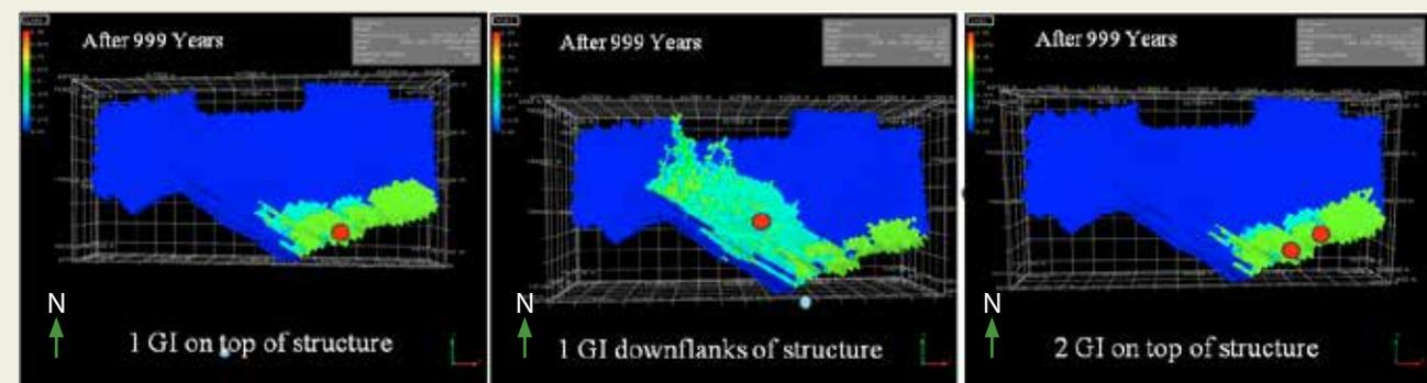
Distribution of injected gas (green) after 1000 years of storage, depending on location of injector well.
