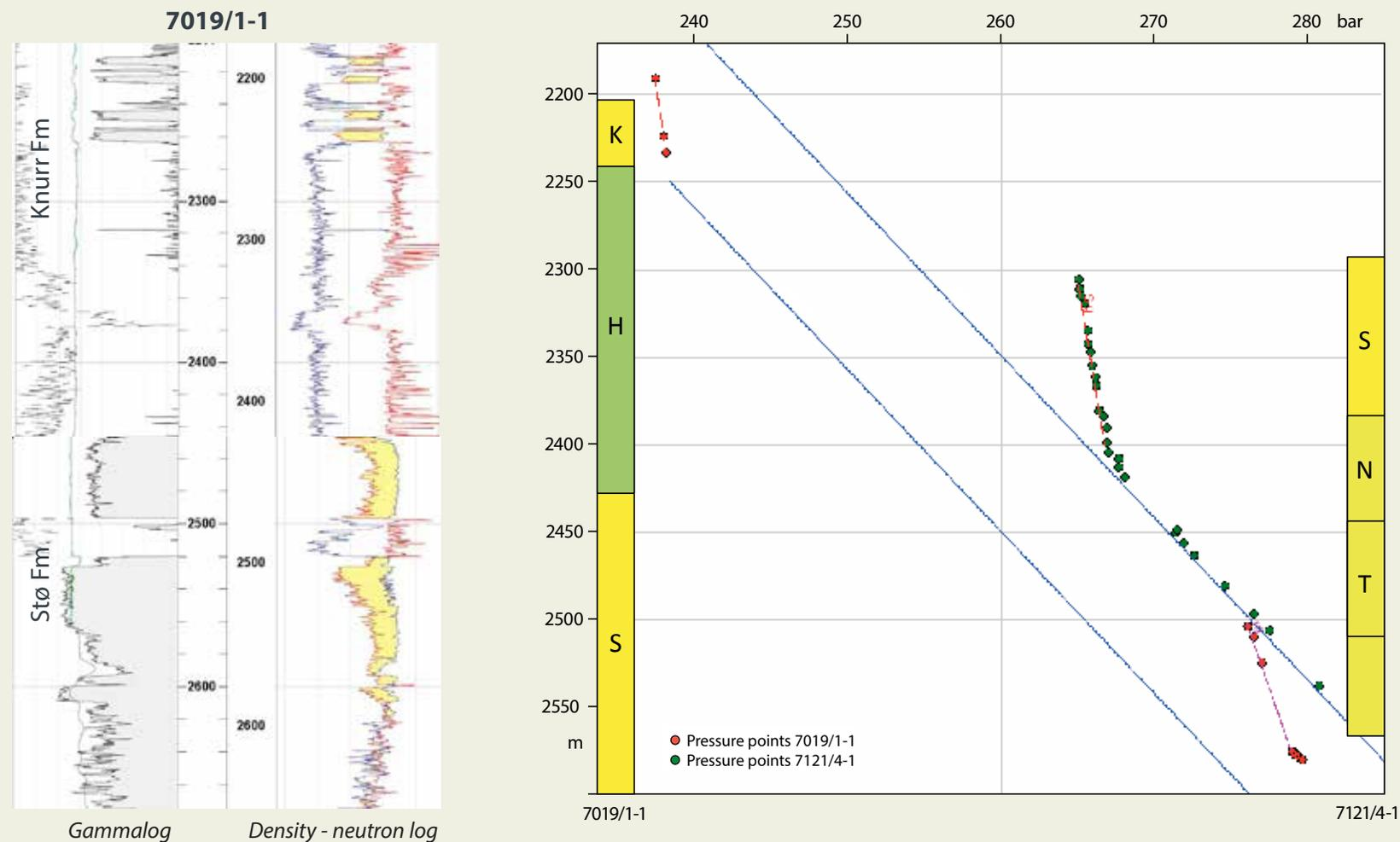
Plot of measured pore pressure in the 7019/1-1 well compared with 7121/4-1 in Snøhvit. Upper blue line: Average water gradient in the Snøhvit area. Lower blue line: Interpreted water gradient in the Cretaceous section of 7019/1-1. Red lines: gas gradients. Color bars show the formation depth in each well. K – Knurr, H – Hekkingen, S – Stø, N – Nordmela, T – Tubåen Formations. Vertical scale: Depth below sea level.
