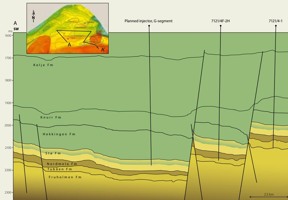
SW-SE profile showing the geometry and thickness variations in the Snøhvit area. Location of CO<sub>2</sub> injection is illustrated. Sealing formations indicated in green color. 7121/4F-2H is the current CO<sub>2</sub> injector.
