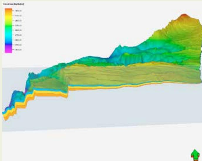
W-E cross section through the Hammerfest Basin 3D geological model, showing the Stø, Nordmela and Tubåen aquifers in blue, yellow and orange respectively.
