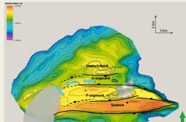
Stø depth map where blue arrows illustrate a possible CO<sub>2</sub> migration after injection in the G segment. Black solid lines illustrate faults with big throw, while black dotted lines indicate where the throw dies out. Grey polygons show location of shallow gas.
