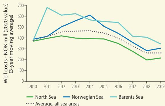
Figure 4.4 Drilling costs per exploration well (well costs) by region, 2010-19
