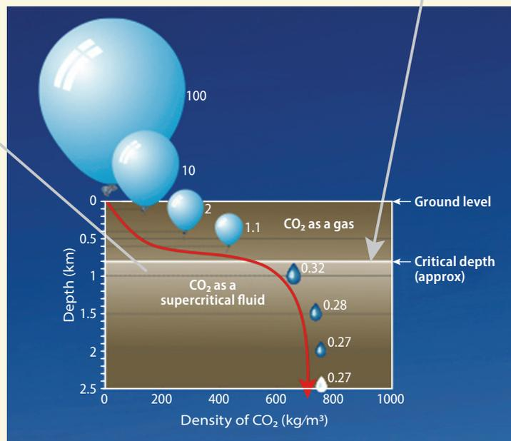
Figure 6.10 Principles for CO<sub>2</sub> storage Source: NPD (2014)
