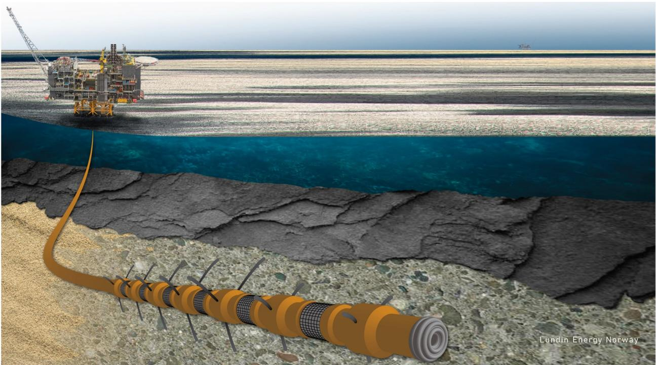
**Figure 3.19 Slim hole drilling**
